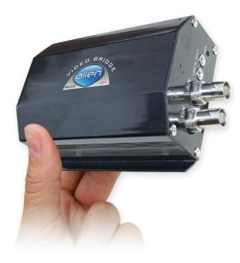
The Video Bridge is a single channel video server and much more! By installing the Bridge at a remote site with an internet connection and power, you are able to view and control a number of devices attached to it via the Internet.
