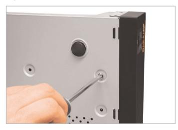
Screw through the four holes in the base of the DVR, and into the four fixing holes in the bottom of the hard drive shown on page 1. (Screws supplied with hard drive.)
