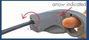
Remove the cable stripper from the co-ax and discard the waste to reveal the prepared co-ax.
