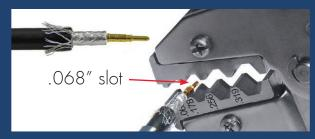
Holding the co-ax, squeeze the crimp tool until the mechanism releases.
