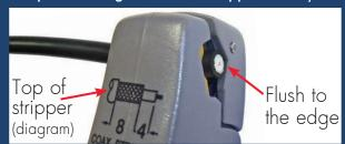
Rotate the cable stripper 2-3 times in the direction indicated on the cable stripper.
