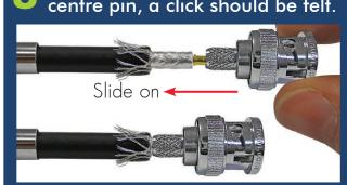
Move the wire braid & ferrule into position over the BNC body.
