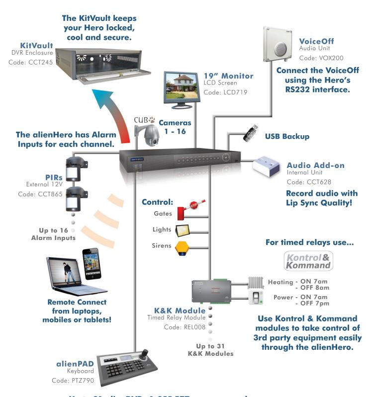
Up to 31 alienDVRs & 255 PTZ cameras can be controlled from just one alienPAD keyboard!
